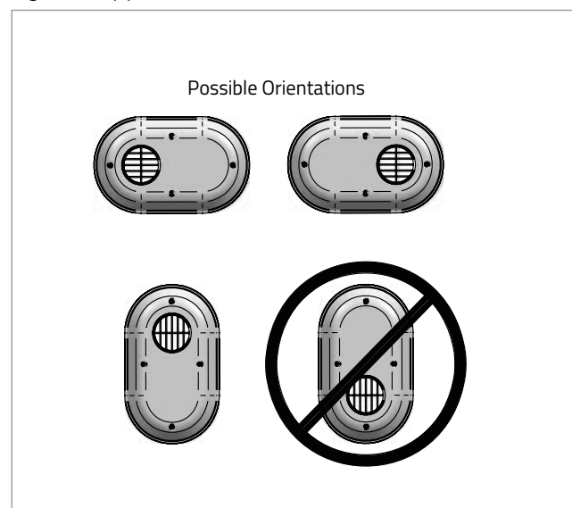
Figure 2: Approved Installation Orientation
