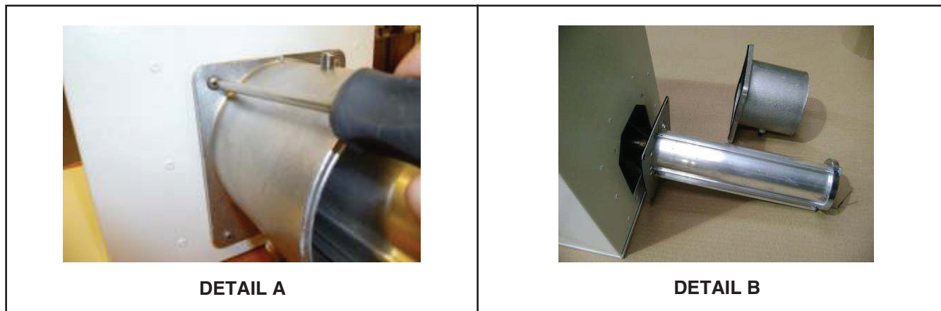
Figure 1. Burner Assembly Removal
