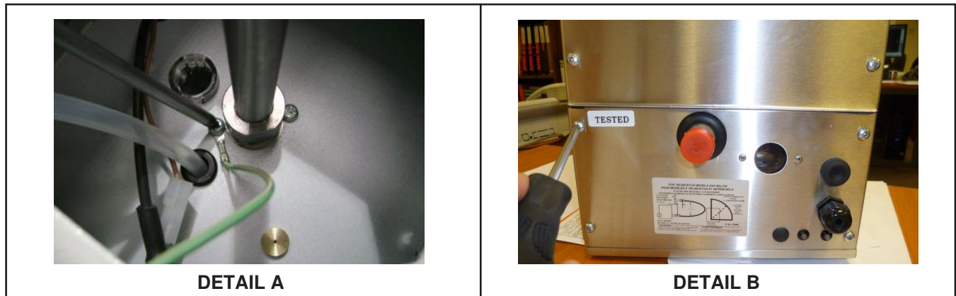
Figure 27. Combination Gas Valve Removal—Models VCS, VCT, and VPT
